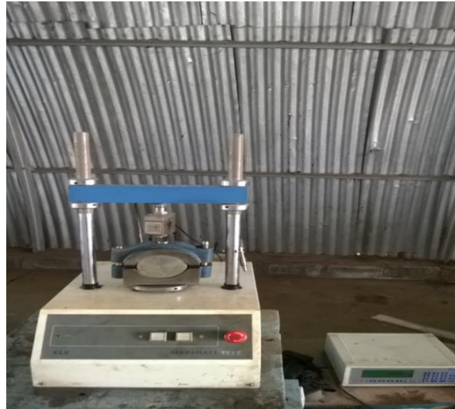
Fig 4: Marshal Test Apparatus
